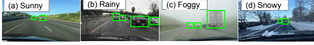
Figure 2: Representative camera frames under sunny, rainy, foggy, and snowy conditions, showing visual degradation in contrast, feature clarity, and object visibility. Green boxes mark detected objects, highlighting how weather variations impact model perception.
