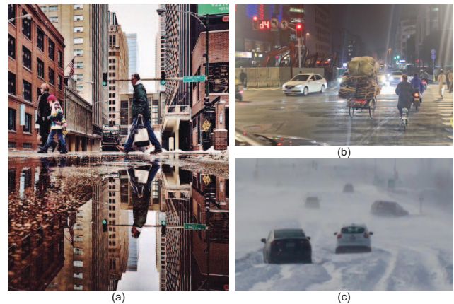
Fig. 1: Scenarios, where AVs fail to accurately analyze, predict, and make decisions, include (a) Road surfaces with standing water [10] which may incorrect positioning of the AV in relation to the image of the water surface. (b) The construction intersection where AVs may fail to predict accurately due to overly complex and unfamiliar scenes. (c) Snow-covered roads where AVs struggle to make correct decisions due to lack of information.
